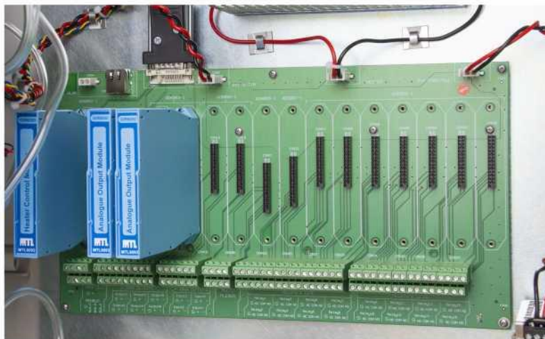
Figure 4.2 - Signal processing motherboard showing connection terminals
